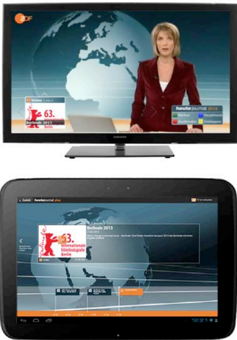
Fig. 4: The synchronized functionality of the 1 st (above) and the 2 nd Screen – on both screens same new content
